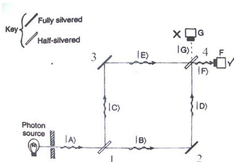
Figure 1. Quantum interferometer. Photon source - a source of photons; Fully silvered - completely reflecting mirror; Half-silvered - a translucent mirror («a divider of photons»); G and F - detectors of photons.
